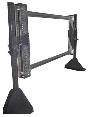
The ability generate controlled, high-intensity electric and magnetic fields over the frequency range of 10 kHz to 100 MHz and a unique design make the EFG-02 the best choice for conducting immunity testing on large, heavy, or bulky DUTs.
