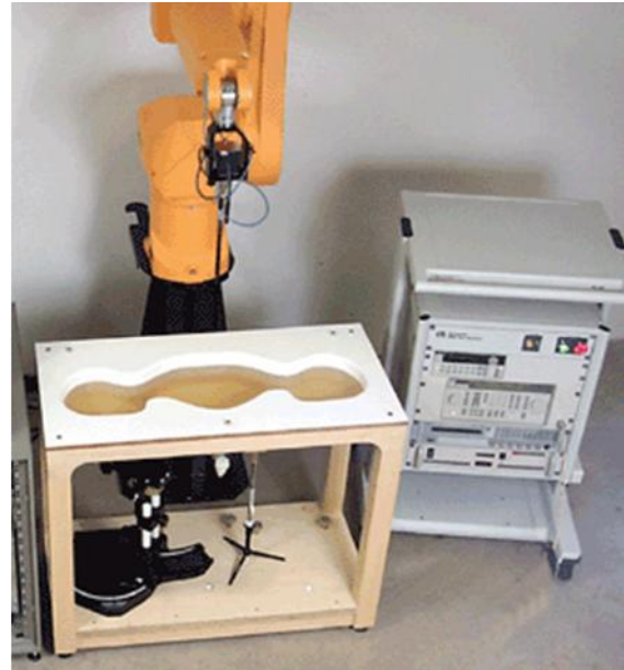
SAR System Components – robot with probe, twin phantom and integrated table, validation instrumentation in mini-rack, dipole antenna, and EUT mounting device.
