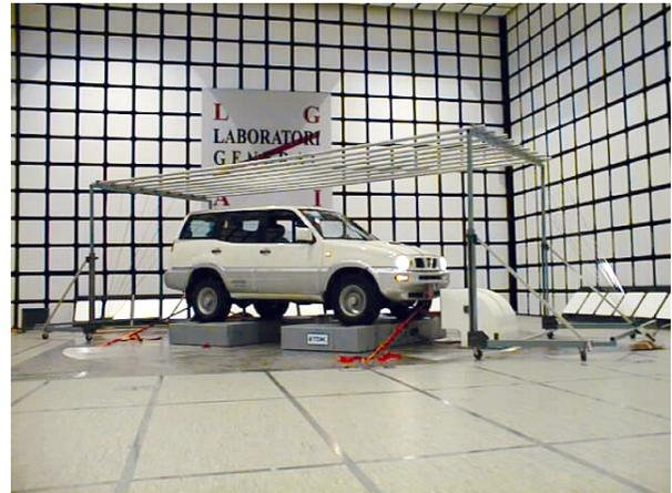
**Figure 2: Stripline for Radiated Immunity Testing**
