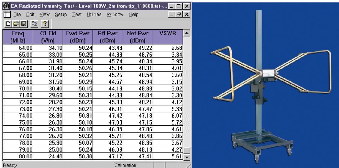
**Figure 3: Software Monitoring the Behavior of a High Power Broadband Antenna**
